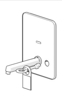
Hang the warning tag plate on the Disinfection Key, insert the Disinfection Key and turn it 180° (direction not important). Place the warning tag in the keys' groove. Activate "Continuous run" Function. See units installation instruction for Sensor Setting Instructions.
